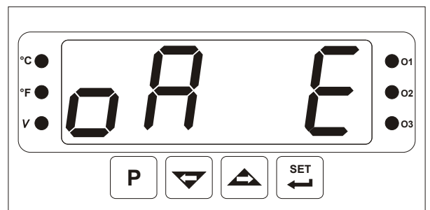
On display which modules are plugged in Module-1 and Module-2 socket is shown. All leds are energised. Above, there is Analog Output on Module-1, Module-2 is empty (Not Used)
