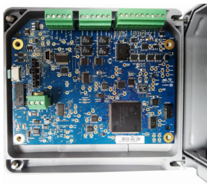
Figure 34: PCB shield removed
