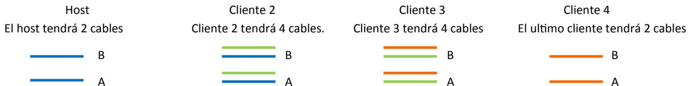
Continue to Daisy Chain until you have tied the chain together, alternating slots on the Daisy Chain until you've reached the end of the chain. The Host and the last Client on the chain will be the only two registers on the chain to have a one wire connection.
