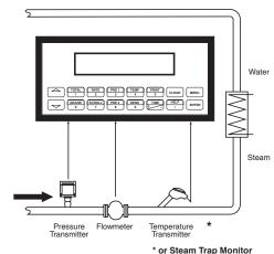
Net Heat Flow = Volume flow • density  $(T, p) \cdot [E_p (T, p) - E_w (T_{S(p)})]$
