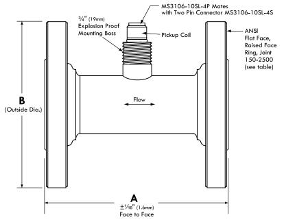
Meter size based on normal inside diameter of pipe. Special flanges can be provided to specification. For hazardous areas, pickup coils with an explosion proof housing can be provided. All flowmeters 5⁄8" and smaller will be provided with 1⁄2" end connections unless otherwise specified.
