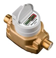
The oscillation is monitored by electrodes placed next to each diffuser wall, in which an electrical current is induced in the jet by a pair of powerful permanent magnets. Sensing electronics capture when the oscillations occur and totalize the volume passed displaying the registered volume on a liquid crystal display.
