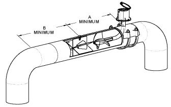
3. Drill a hole (see C dimension in the table). Break line at a flange or cut pipe in a portion near the installation location of the FS100.
