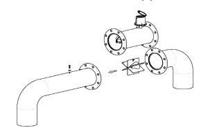
4. Insert the FS100 into the pipe.
