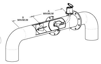
3. Drill a hole (see C dimension in the table). Remove the meter from the line.
