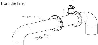
5. Secure the FS100 with the bolt, washer and o-ring supplied with the FS100. Place sealing rubber washer and the o-ring under bolt against the outside of the pipe. Secure the bolt to hold the FS100 to the pipe. Apply Loctite® anti-seize C5-A, or other appropriate lubricant, to the bolt prior to installation to ensure the bolt and nut do not seize up prior to creating an effective seal.
