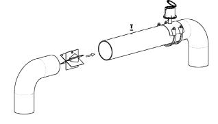
5. Secure the FS100 with the bolt, washer and o-ring supplied with the FS100. Place sealing rubber washer and the o-ring under bolt against the outside of the pipe. Secure the bolt to hold the FS100 to the pipe. Apply Loctite® anti-seize C5-A, or other appropriate lubricant, to the bolt prior to installation to ensure the bolt and nut do not seize up prior to creating an effective seal.
