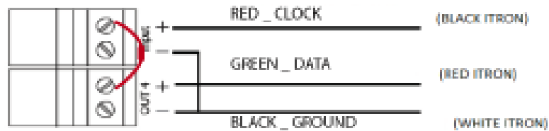
Figure 25: ORION Cellular LTE endpoint connection with resistor
