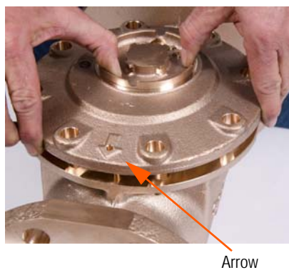
Figure 15 Top Plate Arrow Aligned with Guide Pin
