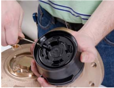
Figure 8 Remove Seal Pin
