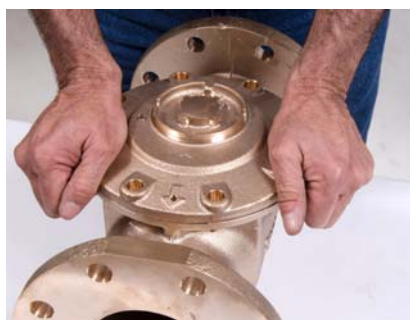
Figure 16 Press Down on Top Plate
