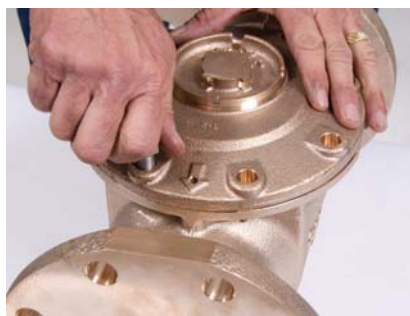
Figure 17 Secure Top Plate with Bolts
