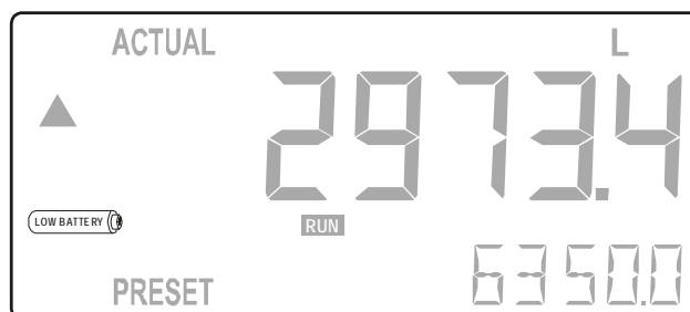
Fig. 6: Example of low-battery alarm.
