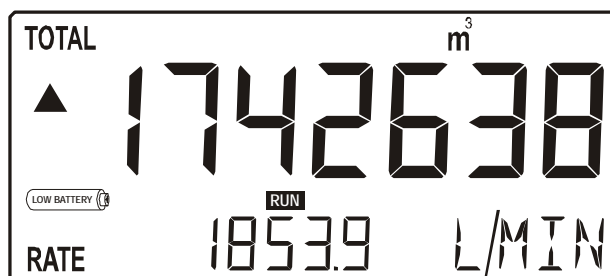
Fig. 5: Example of low-battery alarm
