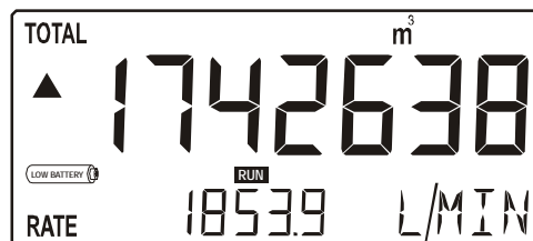
Fig. 4: Example of low-battery alarm.
