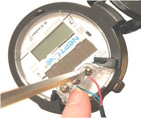
Figure 3: Wiring with Proper Color Wires
