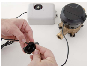
Figure 15: Gray Wires in Slot
